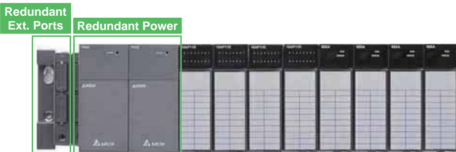
Redundant expansion backplane: AHBP06ER1-5A (6-slot), AHBP08ER1-5A (8-slot)
